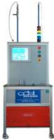
Fig. 34. Device for nondestructive ultrasonic testing of friction welds "opStrut" made by PBP Optel Sp. z o.o. for company BWI in Krosno (Poland)
