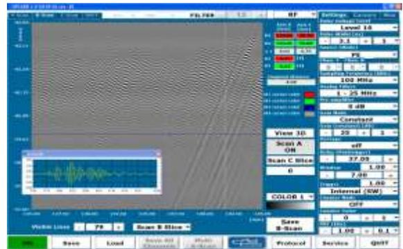
Fig. 33. B- scan for the line with the hole
