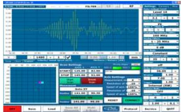
Fig. 32. A- scan. The signal obtained at the point marked with the green marker in Fig. 30
