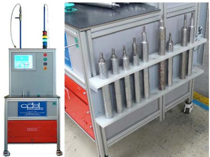
Fig 7. Device for the ultrasonic testing of welds (named *op-Strut*) made by PBP Optel Sp. z o.o for BWI Krosno. Front panel view (a) and the shelf with standard samples (b)
