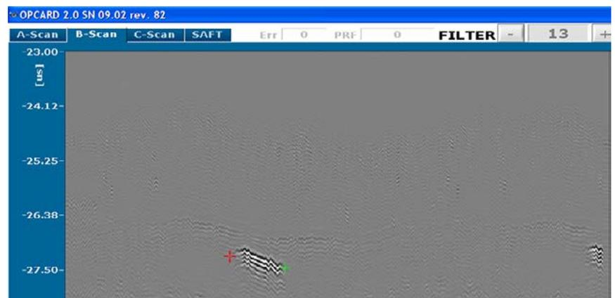
Fig. 15. Two-dimensional visualization of an artificial imperfection presented as B-scan
